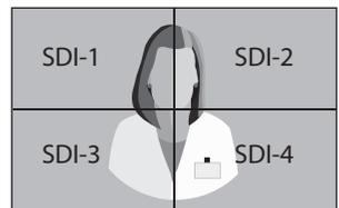
For SDI quad view setting, each connector should correspond with the four image areas as shown above.
